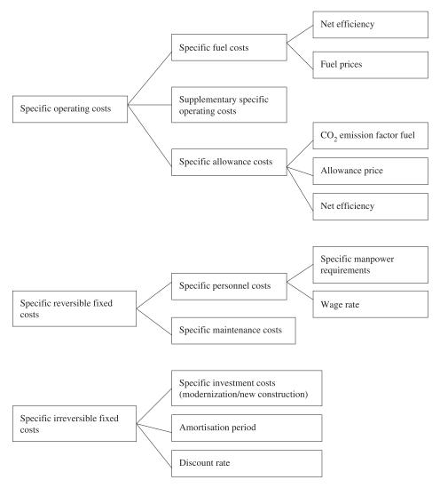
Fig. 2. Determination of cost coefficients.
