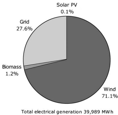
Fig. 2. Annual production of electric energy under the optimal renewable system configuration.
