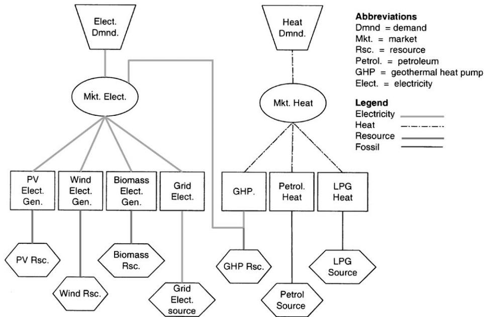
Fig. 1. Network for the renewable energy system in rural area.
