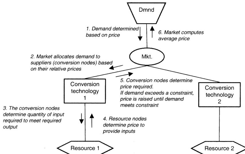
Fig. 9. METANet solution algorithm.
