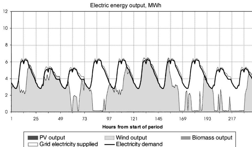
Fig. 3. Electricity generation in early August.
